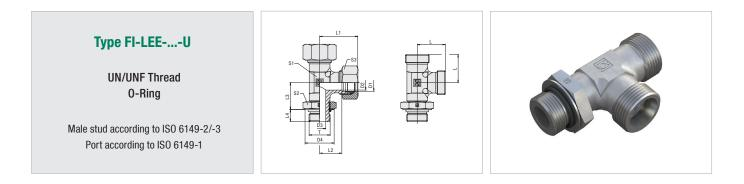
Male threaded studs were designed for female threaded ports in components made of steel. For applications with components made of softer mating materials (e.g. Aluminium), the use of connectors with additionally rolled male threads is recommended.
