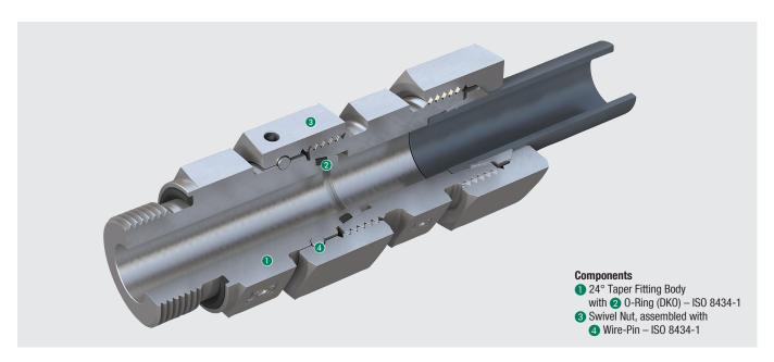
Due to the 24° taper (with o-rings) located on the fitting body itself, STAUFF Connect Tube Fittings with 24° Taper / O-Ring (DKO) represent a logical further development of traditionally available adjustable standpipe tube fittings with factory-assembled cutting rings and union nuts.
