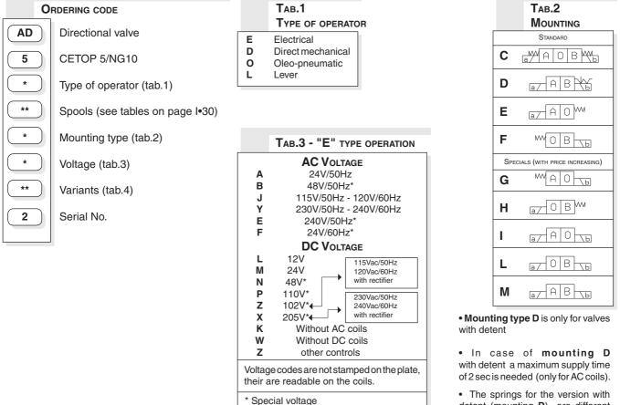
• The springs for the version with detent (mounting **D**) are different from those for standard versions.
