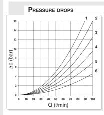
The diagram at the side show the pressure drop curves for spools during normal usage. The fluid used is a mineral oil with a viscosity of 46 mm<sup>2</sup>/s at 40°C; the tests have been carried out at a fluid temperature of  $40^{\circ}$ C.
